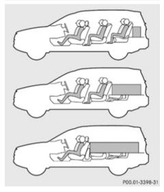
The Gross Vehicle Weight (GVW) which is the weight of the vehicle including fuel, tools, spare wheel, installed accessories. passengers and luggage/cargo must never exceed the load limit and the Gross Vehicle Weight Rating (GVWR) for your vehicle as specified on the placard located on the driver's door B-pillar (⊳ page 275).
