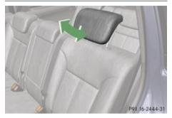
The angle of the head restraint for the outer second-row seats or the third-row seats can be adjusted manually.
