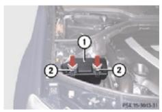
Example illustration fuse box GL 450 (GL 320 BlueTEC, GL 550 similar)
