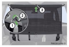
Cargo net installed behind the C-pillar
