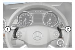
Steering wheel gearshift control (example illustration)
