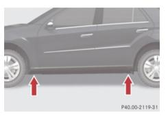
The jack take-up brackets are located directly behind the front wheel housings and in front of the rear wheel housings.
