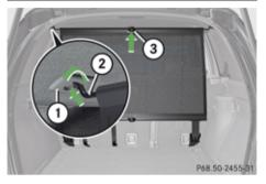
Cargo net installed behind the C-pillar
