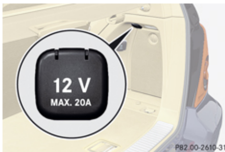
Power outlet in cargo compartment
