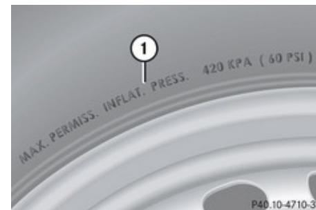
① Maximum permissible tire inflation pressure
