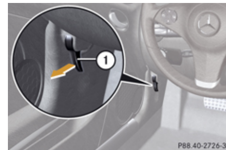
① Hood lock release lever
