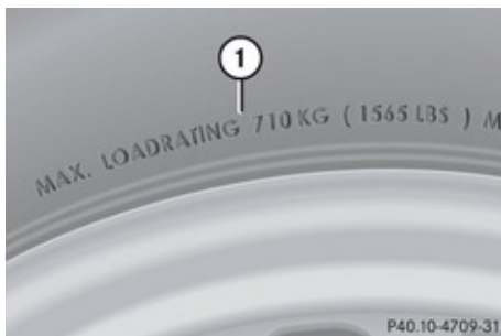
① Maximum tire load rating
