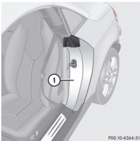
① Driver's door B-pillar
