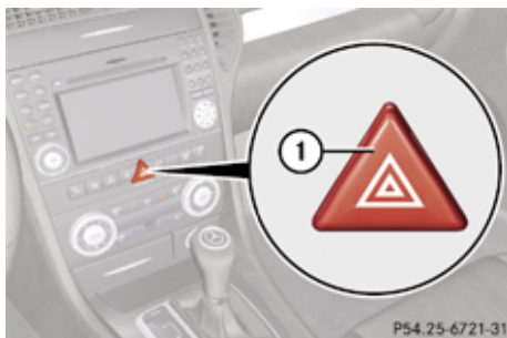
① Hazard warning flasher switch
