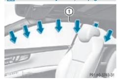
Window curtain air bags (1) are designed to provide increased protection for the head but not the chest or arms.
