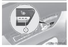
The red indicator lamps in front or rear seat heating button ① come on to show which heating level you have selected.
