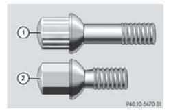
Wheel bolt (1) must be used for light alloy rims. Wheel bolt (2) must be used for the Minispare wheel. The wheel bolts for the Minispare wheel are located in the trunk with the Minispare wheel.
