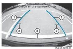
Red guideline (3) indicates an approximate distance of 10 in (0.25 m) from the rear of the vehicle. Yellow guidelines (2) indicate an approximate distance of 3 ft (1 m) from the rear of the vehicle. Blue guidelines (1) indicate the approximate width required for the vehicle.
