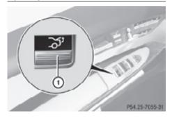
▶ Press and hold remote trunk opening/ closing switch (1) until the trunk begins to open.
