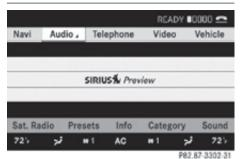
If the satellite radio service has not been activated, only the preview channel is available. You cannot tune in another channel. If you try to do this, you will see the screen described in the section "Satellite radio service is not activated" (▷ page 158).
