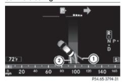
▶ When the vehicle is stationary, turn the steering wheel until red lane ① matches up with yellow lane ②.
