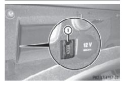
Connect USB storage device to the built-in USB socket ① in the glove box to transfer data (> page 82) or to playback audio tracks (> page 162).
