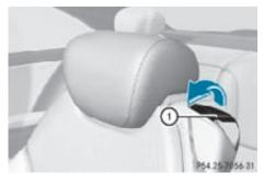
► Folding seat backrest forward: Lift release lever (1) and fold the seat backrest forward.
