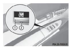
► Activating: Press override switch (1). Indicator lamp (2) comes on.
