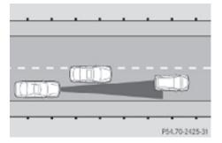
A vehicle traveling in your lane but offset from your direct line of travel may not be detected by the DISTRONIC PLUS. There will be insufficient distance to the preceding vehicle.
