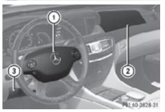
Driver's front air bag ① and front passenger front air bag ② are designed to provide increased protection for the driver and front passenger against the risk of injuries to the head and thorax.
