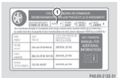
The seating capacity gives you important information on the number of occupants that can be in the vehicle. Observe front and rear seating capacity. The Tire and Loading Information placard showing seating capacity (1) is located on the driver's door
