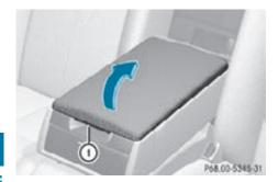
▶ Opening: Pull release catch (1) and swing the storage compartment cover upward in direction of arrow.
