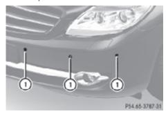
Example illustration, sensors in the front bumper To function properly, sensors ① must be free of dirt, ice, snow and slush. Clean sensors ① regularly. Be careful not to scratch or damage sensors ①, see "Cleaning the driving systems sensors" (> page 406).
