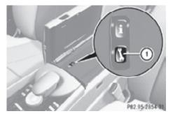
▶ Press and hold Roadside Assistance button (1) for longer than 2 seconds. A call to a Mercedes-Benz Roadside Assistance dispatcher will be initiated. The indicator lamp in Roadside Assistance button (1) will flash while the call is in progress. The message Connecting
