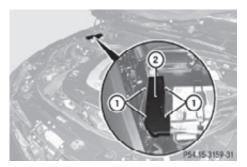
Example illustration fuse box on passenger side
