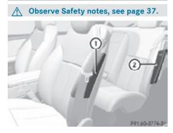
Front side impact air bags (1) and rear side impact air bags (2) are designed to provide increased protection for the thorax but not the head, neck and arms.
