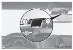
▶ Use recessed handles (1) of camera cover to swing camera cover downward.
