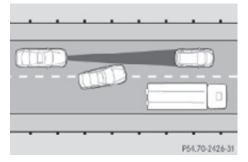
The DISTRONIC PLUS has not yet detected the vehicle changing lanes. There will be insufficient distance to the lane-changing vehicle.
