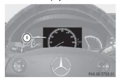
For example, telephone numbers are shown in the multifunction display (1) while dialing when the main Telephone menu is selected in the instrument cluster control system.
