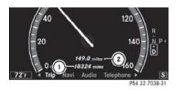
In the standard display, the main odometer ① and the trip odometer ② appear in the multifunction display.
