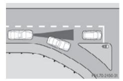
The DISTRONIC PLUS does not brake for obstacles or stationary vehicles. If, for example, the vehicle detected in front of you changes lanes to bypass an obstacle or stationary vehicle in front of it, the DISTRONIC PLUS will not brake for the obstacle or stationary vehicle.
