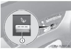
The blue indicator lamps in seat ventilation button ① come on to show which ventilation level you have selected.
