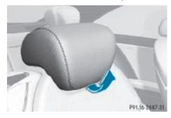
▶ Push or pull on the lower edge of the head restraint cushion to the desired position.
