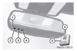
Interior rear view mirror with integrated remote
