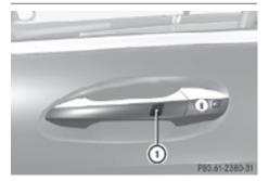
The SmartKey with KEYLESS-GO must be located outside the vehicle within approximately 3 ft (1 m) of a door.
