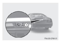
Camera lens (1) must be free of dirt, ice, snow, and slush to function properly. Clean the camera lens regularly. Being careful not to scratch or damage the camera lens, see "Cleaning the rear view camera lens" (⊳ page 407).
