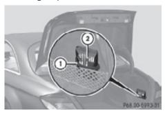
► Loosen tensioning strap ①. First aid kit ② can be removed.
