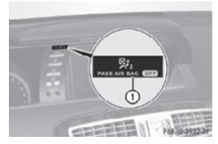
PASS AIR BAG III indicator lamp (1) will be illuminated, except with the SmartKey removed from the starter switch or with the starter switch in position **0**.
