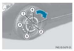
► Tighten the five wheel bolts evenly, following the diagonal sequence illustrated (1) to (5), until all bolts are tight. Observe a tightening torque of 110 lb-ft (150 Nm).
