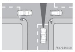
The DISTRONIC PLUS may inadvertently detect crossing vehicles. If you switch on the DISTRONIC PLUS, for example, at a traffic light with cross traffic, the vehicle may suddenly start to drive off.
