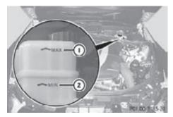
The brake fluid level is correct when it is between lower mark (MIN) ② and upper mark (MAX) ① of the brake fluid reservoir.
