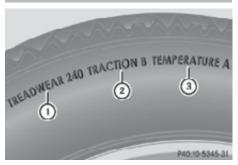
Government requirement designed to give drivers consistent and reliable information regarding tire performance. Tire manufacturers are required to grade tires based on three performance factors: treadwear ①, traction ②, and temperature resistance ③. Although not a Government of Canada requirement, all tires made for sale in North America have these grades branded on the sidewall.
