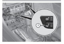
The blue indicator lamps in seat ventilation switch (1) come on to show which ventilation level you have selected.
