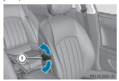
Move adjustment lever ① in direction of the arrows until you have reached a comfortable seating position.
