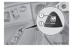
► Activating: Press override switch ①. Indicator lamp ② comes on.
