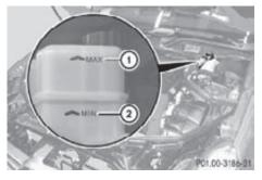
The brake fluid level is correct when it is between lower mark (MIN) (2) and upper mark (MAX) (1) of the brake fluid reservoir.
