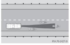
Because of their narrow profile, the vehicles traveling near the outer edges of the lane have not yet been detected by the Distronic. There will be insufficient distance to the preceding vehicles.
