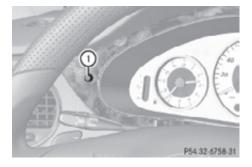
➤ Clearing the maintenance service indicator message manually: Press reset button ① on the instrument cluster.
