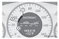
When the Distronic detects a vehicle directly ahead, the cruise control speed segments ② appear in the speedometer. These segments represent the difference between the set speed of your vehicle ① and the speed of the preceding vehicle ③.
