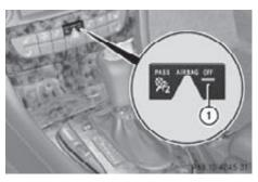
PASS AIR BAG OFF [ ] indicator lamp ① will be illuminated, except with the SmartKey removed from the starter switch or with the starter switch in position **0**.
