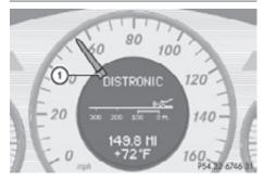
When the Distronic is activated, one or two cruise control speed segments come on around set speed (1).
