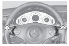
Steering wheel gearshift control (example illustration)
