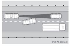
The Distronic has not yet detected the vehicle changing lanes. There will be insufficient distance to the lane-changing vehicle.
