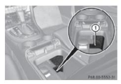
► Opening/closing air vent: Slide lever ①
