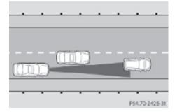
A vehicle traveling in your lane but offset from your direct line of travel may not be detected by the Distronic. There will be insufficient distance to the preceding vehicle.
