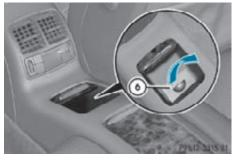
With insert or cup holder removed, fold cover (a) upward in direction of arrow.
