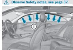
Window curtain air bags ① are designed to provide increased protection for the head but not the chest or arms.
