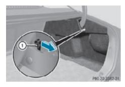
▶ Pull fuel filler flap release ① in direction of arrow.
