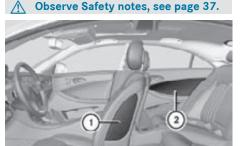
Front side impact air bags ① and rear side impact air bags ② are designed to provide increased protection for the thorax but not the head, neck and arms.
