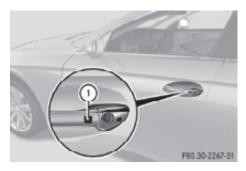
► **Global locking:** Press lock button ① on an outside door handle.
