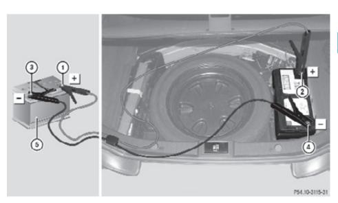
Position (5) represents the charged battery of another vehicle or an equivalent starter pack.
