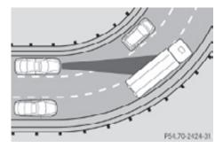
In turns or bends, the Distronic may not detect a moving vehicle in front, or it may detect one too soon. This may cause your vehicle to brake late or unexpectedly.
