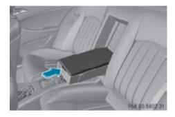
▶ Opening: Press the handle upwards and fold the rear armrest lid up.
