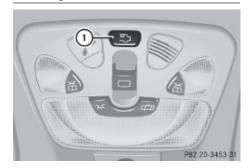
► Switching rear interior lamp on/off: Press switch (1).
