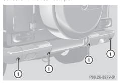
To function properly, sensors (1) must be free of dirt, ice, snow and slush. Clean sensors (1) regularly, being careful not to scratch or damage sensors (1), see "Cleaning the Rear Parking Assist system sensors" (⊳ page 195).
