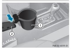
▶ Place bracket of cup holder (1) into recess indicated by arrow of cup holder base (2). If the cup holder is no longer in use, it can for example, be stored in the glove box or storage compartment below the armrest.
