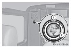
The warning indicator is divided into four yellow and two red distance segments ①. The Rear Parking Assist system is ready to measure when you hear a signal and readiness indicator ② is illuminated.
