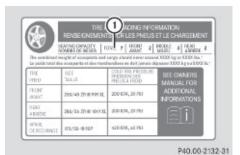
The seating capacity gives you important information on the number of occupants that can be in the vehicle. Observe front and rear seating capacity. The Tire and Loading Information placard showing seating capacity ① is located on the driver's door B-pillar (> page 166).
