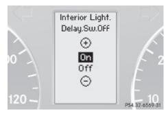
▶ Press button + or - to switch the interior lighting delayed shut-off feature 0n or 0ff.
