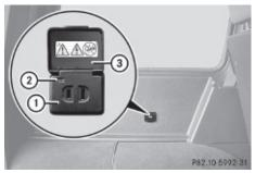
The 115V AC socket (1) provides an alternating current of 115 volts, which enables you to connect small electrical devices with a combined received power of 150 W at most. You can connect small devices such as game consoles, mobile phone chargers, laptops, etc.
