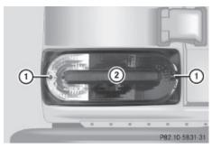
Example illustration: Left tail lamp lens (right tail lamp lens laterally reversed)
