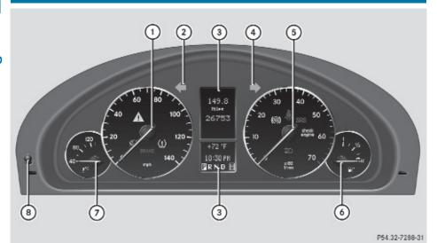
**Function Page** (5) Tachometer with: Antilock Brake
