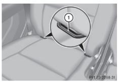
LATCH-type (ISOFIX) anchors (1) are located between the seat cushion and the backrest.
