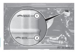
The brake fluid level is correct when it is between lower mark (MIN) (2) and upper mark (MAX) (1) of the brake fluid reservoir.
