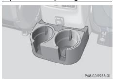
■ Before folding the rear seat backrest and the rear seat bench forward, make sure that all containers in the rear cup holder are removed.
