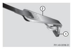
▶ For safety, make sure hook ② is attached to anchorage ring (1) beyond the safety catch, as illustrated.
