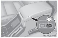
▶ Press and hold Roadside Assistance button (1) for longer than 2 seconds. A call to a Mercedes-Benz Roadside Assistance dispatcher will be initiated. The indicator lamp in Roadside Assistance button (1) will flash while the call is in progress. The message Connecting Call will appear in the multifunction display and the COMAND system is muted.
