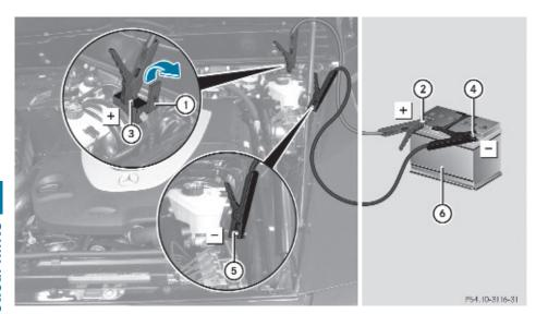
Position (6) represents the charged battery of another vehicle or an equivalent starter pack.
