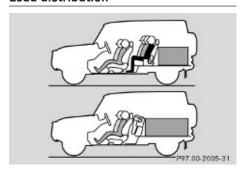
The Gross Vehicle Weight (GVW) is the weight of the vehicle including:
