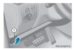
▶ Pull hood lock release lever (1). The hood is unlocked.
