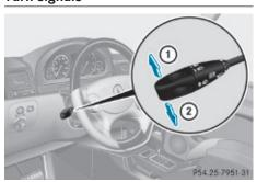
▶ Press the combination switch in direction of arrow ① or ②.
