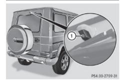
▶ Only use clean water and a soft, nonscratching cloth to clean rear view camera lens ①. Be careful not to apply wax to rear view camera lens ① when waxing the vehicle. If necessary, remove the wax using the Mercedes-Benz approved Car Shampoo with plenty of water.
