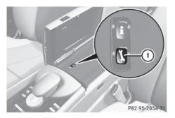
▶ Press and hold Roadside Assistance button ① for more than two seconds. A call to a Mercedes-Benz Roadside Assistance Representative is initiated. The indicator lamp in Roadside Assistance button ① flashes while the call is active. The Connecting Call message appears in the COMAND display and COMAND is muted.
