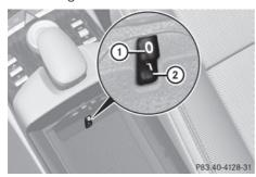
► To switch the ventilation on/off: push rocker switch down ② or up ①.
