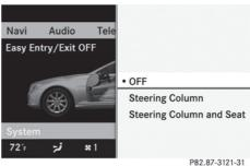
▶ To set the EASY-ENTRY/EXIT feature: select Vehicle in the main function bar by sliding ← ○ → and turning 【 ○ 】 the
