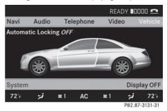
► To switch the automatic locking feature on/off: select Vehicle in the main function bar by sliding ← → and
