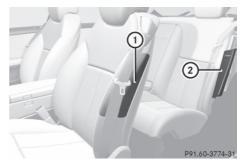
Front side impact air bags (1) and rear side impact air bags (2) are deployed next to the outer seat cushions.
