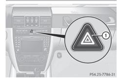
The hazard warning lamp switches on automatically if an air bag or the belt tensioners are triggered and the SmartKey is in position 1 in the ignition lock.
