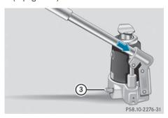
► Turn pressure release screw (3) clockwise as far as it will go using notch (2) on the pump lever.
