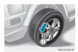
▶ Using lug wrench (1), loosen the bolts on the wheel you wish to change by about one full turn. Do not unscrew the wheel bolts completely.
