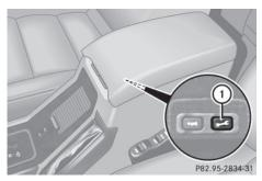
▶ Press and hold Roadside Assistance button ① for more than two seconds. A call to a Mercedes-Benz Roadside Assistance Representative is initiated. The indicator lamp in Roadside Assistance button ① flashes while the call is active. The Connecting call message appears in the multifunction display and the COMAND system is muted.
