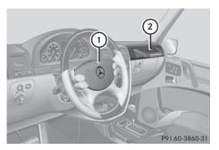
Driver's air bag (1) deploys in front of the steering wheel; front-passenger front air bag (2) deploys in front of and above the glove box.
