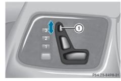
▶ Slide head restraint adjustment button (1) up or down in the direction of the arrow.
