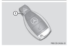
▶ Press the 🔒 or 🗊 button. The SmartKey battery is working properly if battery check lamp (1) lights up briefly.
