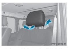
▶ Push or pull the lower edge of the head restraint in the direction of the arrow.
