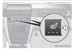
1 The system automatically switches down from level 3 to level 2 after approximately five minutes.
