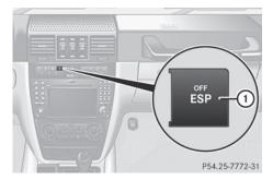
▶ To deactivate: press button (1) until the warning lamp lights up in the instrument cluster.
