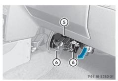
To make it easier to change the fuse, you can fold fuse box (5) down slightly:
