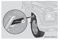
VIN (stamped into the chassis on the right-hand side, when viewed in the direction of travel)
