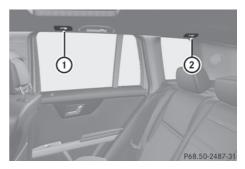
• The brackets behind B-pillar ① are required for the cargo compartment enlargement (▷ page 208).
