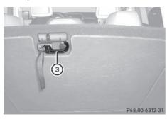
Release hook ③ from the bracket on the underside of the trunk floor.
