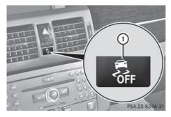
► To deactivate: press button ①. The Green warning lamp in the instrument cluster lights up.
