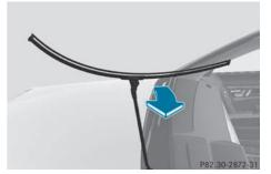
Remove the wiper blade from the retainer on the wiper arm in the direction of the arrow.
