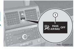
If the SmartKey has been removed from the ignition lock or is in position  $\mathbf{0}$ , indicator lamp  $\mathbf{1}$  (1) does not light up.
