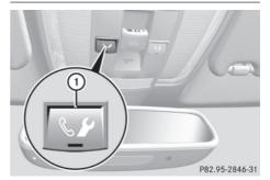
Press and hold Roadside Assistance button ① for more than two seconds. A call to a Mercedes-Benz Roadside Assistance Representative is initiated. The indicator lamp in Roadside Assistance button ① flashes while the call is active. The Connecting Call message appears in the multifunction display and the audio system or COMAND is muted.
