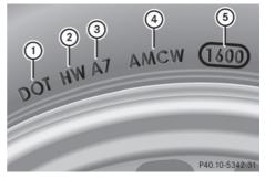
The TIN is a unique identification number. The TIN enables the tire manufacturers to inform purchasers of recalls and other safetyrelevant matters. It makes it possible for the purchaser to easily identify the affected tires. The TIN is made up of manufacturer
