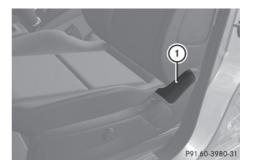
Pelvis air bags ① deploy next to and below the outer seat cushions. They are deployed:
