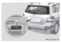
On vehicles with the EASY-PACK tailgate: if you pull handle (1) and keep it in this position, you can open the tailgate manually. If you release the handle, the tailgate automatically opens fully.
