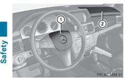
Driver's air bag ① deploys in front of the steering wheel; front-passenger air bag ② deploys in front of and above the glove box. They are deployed:
