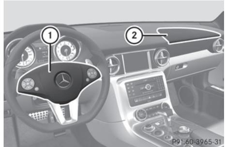
Driver's front air bag ① and passenger front air bag ② are designed to provide increased protection for the driver and passenger against the risk of injuries to the head and thorax.
