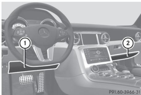
Driver side knee bag ① is located on the driver side lower instrument panel. Passenger side knee bag ② is located on the passenger side below the glove box. They are designed to operate together with the front air bags in certain frontal impacts if the system
