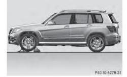
Securing the vehicle on level ground
