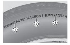
Uniform Tire Quality Grading Standards are U.S. government specifications. Their purpose is to provide drivers with uniform reliable information on tire performance data. tire manufacturers have to grade tires using three performance factors: tread wear (1), tire traction (2) and heat resistance (3). All tires sold in North America are provided with the corresponding quality class mark on the sidewall of the tire, even though these regulations do not apply to Canada.
