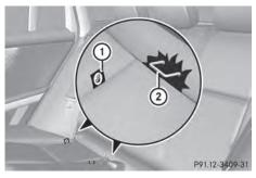
Installation instructions ① indicate the installation location of securing rings ②.
