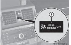
If the SmartKey has been removed from the ignition lock or is in position **0**, the **2 Description** indicator lamp (1) does not light up.
