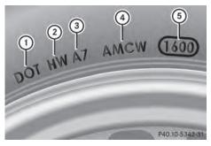
The TIN is a unique identification number. The TIN enables tire manufacturers to inform purchasers of recalls and other safetyrelevant matters. It makes it possible for the purchaser to easily identify the affected tires. The TIN is made up of manufacturer identification code (2), tire size (3), tire type code (4) and manufacturing date (5).
