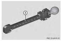
Re-insert lever extension (2) downwards (swelling) with guide rail (3).
