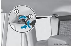
Cargo net installed behind the C-pillar
