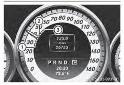
When DISTRONIC PLUS is activated, one or two segments (2) in the set speed range light up.
