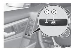
▶ To activate/deactivate: press button ②. If indicator lamp ① is lit, operation of the rear side windows is disabled. Operation is only possible using the switches in the driver's door. If indicator lamp ① is off, operation is possible using the switches in the rear compartment.
