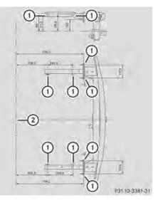
Anchorage points for the trailer tow hitch (example)
