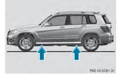
The jacking points are located just behind the wheel housings of the front wheels and just in front of the wheel housings of the rear wheels (arrows).
