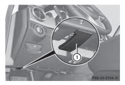
Pull release lever ① on the hood. The hood is released.
