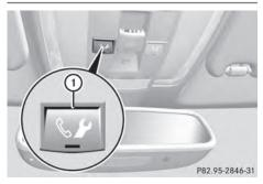
Press Roadside Assistance button (1). This initiates a call to the Mercedes-Benz Customer Assistance Center. The indicator lamp in Roadside Assistance button (1) flashes while the call is active. The Connecting Call message appears on the multifunction display. The audio output is muted.
