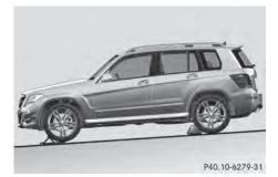
Securing the vehicle on slight downhill gradients
