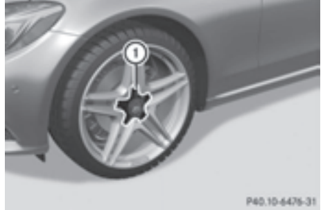
Alloy wheel with plastic hub cap
