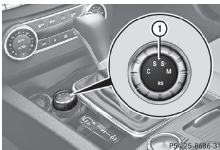
Drive program selector with manual drive program
