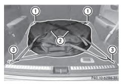
In vehicles with a Bang & Olufsen sound system, the "Minispare" emergency spare wheel is stored in a bag. The bag is secured to the cargo tie-down rings in the cargo compartment.
