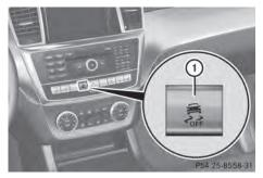
► To switch off: press button ①. The SFF ESP<sup>®</sup> OFF warning lamp in the instrument cluster lights up. ► To switch on: press button ①. The SFE ESP® OFF warning lamp in the instrument cluster goes out.
