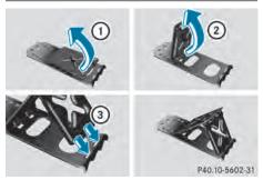
If your vehicle is equipped with a wheel chock, it can be found in the tire-change tool kit (> page 382). The folding wheel chock is an additional securing measure to prevent the vehicle from rolling away, for example when changing a wheel.
