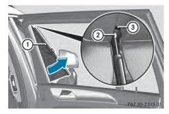
The roller sunblind can be hooked back into place should it pop out from the top of the guide rail.
