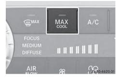
MAX COOL is only operational when the engine is running.
