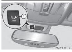
Press Roadside Assistance button ①. This initiates a call to the Mercedes-Benz Customer Assistance Center. The indicator lamp in Roadside Assistance button ① flashes while the call is active. The Connecting Call message appears on the multifunction display. The audio output is muted.
