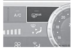
The rear window defroster has a high current draw. You should therefore switch it off as soon as the rear window is clear. Otherwise, the rear window defroster switches off automatically after several minutes.
