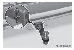
Correctly installed and secured ball coupling
