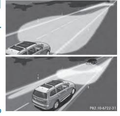
You can use this function to set the headlamps to change between low beam and high beam automatically. The system recognizes vehicles with their lights on, either approaching from the opposite direction or traveling in front of your vehicle, and consequently switches the headlamps from high beam to low beam.
