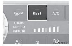
It is possible to make use of the residual heat of the engine to continue heating the stationary vehicle for up to 30 minutes after the engine has been switched off. The heating time depends on the temperature that has been set.
