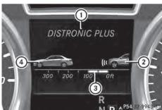
Distance display with DISTRONIC PLUS activated in the multifunction display
