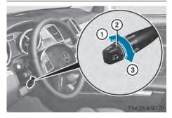
You can set the specified minimum distance for DISTRONIC PLUS by varying the time span between one and two seconds. With this function, you can set the minimum distance that DISTRONIC PLUS keeps to the vehicle in front, dependent on vehicle speed. You can see this distance in the multifunction display (> page 205).
