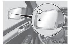
If you switch on the turn signals to change lanes and a vehicle is detected in the side monitoring range, you receive a visual and acoustic collision warning. You then hear a double warning tone and red warning lamp ① flashes. If the turn signal remains on, detected vehicles are indicated by the flashing of red warning lamp ①. There are no further warning tones.
