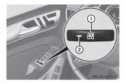
► To activate/deactivate: press button (1). If indicator lamp (2) is lit, operation of the rear side windows is disabled. Operation is only possible using the switches in the driver's door. If indicator lamp ② is off, operation is possible using the switches in the rear compartment.
