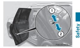
You secure each door individually with the child-proof locks on the rear doors. A door secured with a child-proof lock cannot be opened from inside the vehicle. When the vehicle is unlocked, the door can be opened from the outside.
