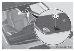
Active Lane Keeping Assist monitors the area in front of your vehicle by means of
