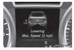
If you maintain or reduce your speed, you will see a message in white in the display while the vehicle is being lowered, such as the following: Vehicle Lowering Max. Speed 12 mph (20 km/h).
