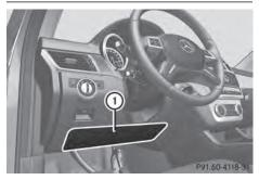
Driver's knee bag ① deploys under the steering column. The driver's knee bag is always deployed along with the driver's front air bag. The driver's knee bag is designed to operate together with the front air bags in frontal impacts if certain thresholds are exceeded. The driver's knee bag operates best in conjunction with correctly positioned and fastened seat belts.
