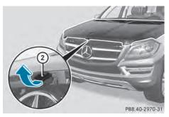
Reach into the gap, pull hood catch handle (2) up and lift the hood.
