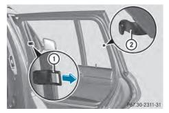
► To extend: pull the roller sunblind out by tab (1) and hook it onto retainers (2) at the back of the window.
