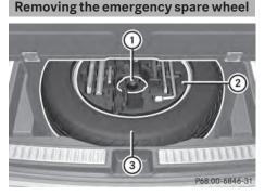
Emergency spare wheel (example: vehicle without lockable cargo compartment floor)
