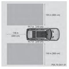
Active Blind Spot Assist monitors the area up to 10 ft (3.0 m) behind your vehicle and directly next to your vehicle, as shown in the diagram. For this purpose, Active Blind Spot Assist uses radar sensors in the rear bumper.
