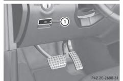
► While driving, push handle ① of the electric parking brake.
