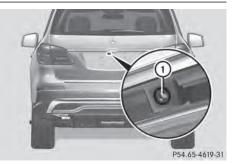
Rear view camera 1 is in the handle on the tailgate.
