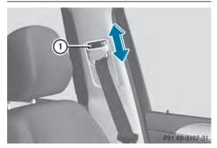
You can adjust the seat belt height on the front seats. Adjust the belt to a height that allows the upper part of the seat belt to be routed across the center of your shoulder.
