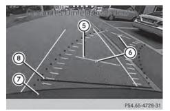
(5) Yellow guide line at a distance of approximately 3 ft (1.0 m) from the rear of the vehicle
