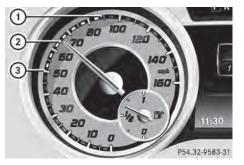
Example: DISTRONIC PLUS displays in the speedometer
