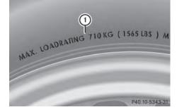
Maximum tire load (1) is the maximum permissible weight for which the tire is approved.
