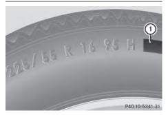
In addition to the load bearing index, load index (1) may be imprinted after the letters that identify the speed index (6) on the sidewall of the tire ( $\triangleright$  page 417).
