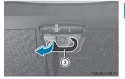
► Fold out hook ③ on the underside of the cargo compartment floor in the direction of the arrow.
