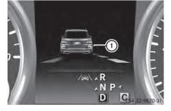
If a lane-correcting brake application occurs, display (1) appears in the multifunction display.
