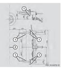
Anchorage points for the trailer tow hitch (example)
