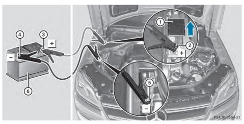
Position number (6) identifies the charged battery of the other vehicle or an equivalent jumpstarting device.
