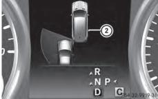
If Active Blind Spot Assist detects a risk of a lateral collision in the monitoring range, a course-correcting brake application is carried out. This is meant to assist you in avoiding a collision.
