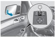
① To fold the exterior mirrors in or out
