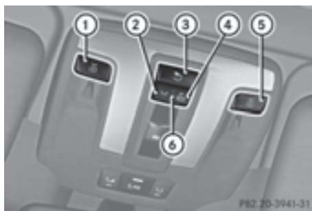
Front overhead control panel
