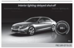
The interior lighting is activated for the duration of the delayed switch-off time when the SmartKey is removed from the ignition lock.
