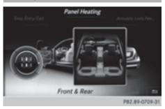
The panel heating function warms the surfaces with which the vehicle occupants frequently come into contact. Activation of the panel heating using COMAND as described below only works if seat heating is activated (see the vehicle Operator's Manual).
