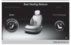
The balance function controls the distribution of heat on the seat backrest and cushion.
