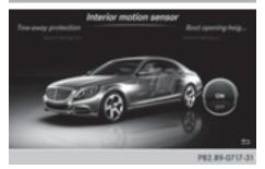
When the interior motion sensor is armed, a visual and audible alarm is triggered if movement is detected in the vehicle interior. This can occur if someone reaches into the vehicle interior without authorization, for example.
