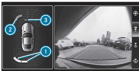
Parking Assist PARKTRONIC warning display (vehicles with front and rear view camera)
