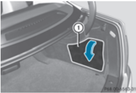
Right-hand side trim panel
