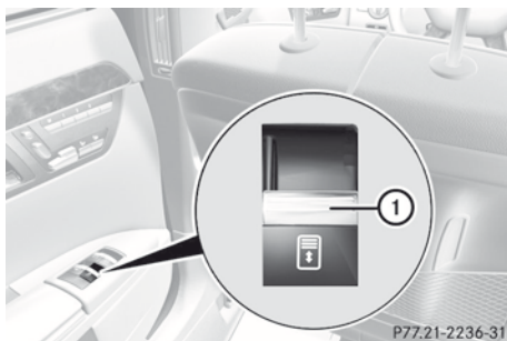
Door control panel in rear
