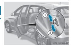
You secure each door individually with the child-proof locks on the rear doors. A door secured with a child-proof lock cannot be opened from inside the vehicle. When the vehicle is unlocked, the door can be opened from the outside.
