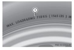
Maximum tire load ① is the maximum permissible weight for which the tire is approved.
