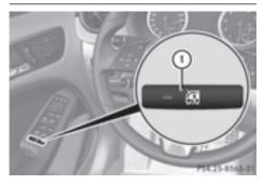
► To activate/deactivate: press button ①. If indicator lamp is lit, operation of the rear side windows is disabled. Operation is only possible using the switches in the driver's door. If the indicator lamp is off, operation is possible using the switches in the rear compartment.
