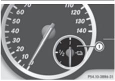
Condition of charge display ① shows the condition of charge of the high-voltage battery. The charge values are shown as a percentage in the COMAND display (see the separate operating instructions).
