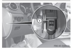
Your vehicle is equipped with a high-voltage switch-off device (1) which can be used to switch off the vehicle's high-voltage electrical system.
