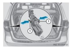
Press retaining lugs ① simultaneously in the direction of the arrow and pull the bulb holder out.
