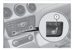
The three red indicator lamps in the button indicate the heating level you have selected. The system automatically switches from level **3** to level **2** after approximately eight minutes.
