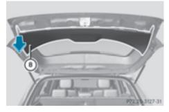
► Unclip part of trim ⑧ from the assembly using a sudden, sharp movement, until bulb holder ⑨ is accessible.
