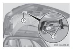
Remove bulb holder (9) using both sides of lever (10).
