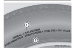
This information describes the type of tire cord and the number of layers in sidewall (1) and under tire tread (2).
