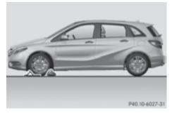
Securing the vehicle on level ground
