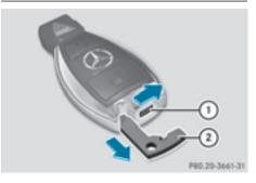
Push release catch ① in the direction of the arrow and at the same time remove mechanical key ② from the SmartKey.
