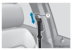
The shoulder section of the seat belt must always be routed across the center of the shoulder. Adjust the belt outlet if necessary.
