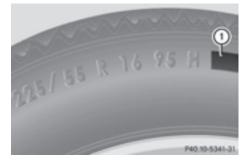
In addition to the load bearing index, load index (1) may be imprinted after the letters that identify speed index (3) on the sidewall of the tire ( $\triangleright$  page 293).
