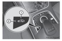
It is possible to choose between the "Normal" and "Raised" vehicle levels. Select the "Normal" setting for normal road surfaces and "Raised" for driving with snow chains or on particularly poor road surfaces. Your selection remains stored even if you remove the SmartKey from the ignition lock.
