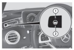
Press button ②. Indicator lamp ① goes out. The DTR+: Steering Assist. Off message appears in the multifunction display. Steering Assist and Stop&Go Pilot are deactivated.
