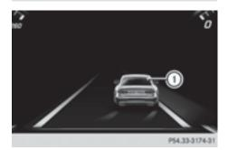
If a lane-correcting brake application occurs, display (1) appears in the multifunction display. The brake application also slightly reduces vehicle speed.
