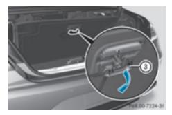
► Fold out hook ③ on the underside of the trunk floor.
