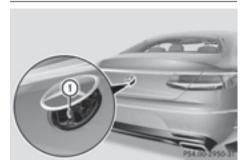
Rear view camera ① is under a flap in the trunk lid.
