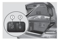
Press and release closing button ① on the trunk lid.
