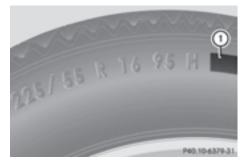
In addition to the load-bearing index, load index (1) may also be imprinted on the side-wall of the tire. You will find this after the let-
