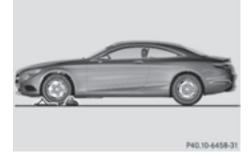
On level ground: place chocks or other suitable items under the front and rear of the wheel that is diagonally opposite the wheel you wish to change.
