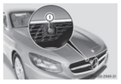
Camera lens ① is cleaned at regular intervals by operating the windshield washer system.
