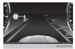
Pedestrian symbol ① in the assistance graphic indicates the status of the spotlight function. If the symbol is displayed not filled in, the function is switched on. If the symbol is displayed filled in, the conditions for the spotlight function are met.
