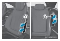
Front side impact air bags (1) and rear side impact air bags (2) deploy next to the outer bolster of the seat backrest.
