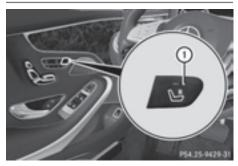
The SmartKey must be in the ignition lock and in position 1 or 2, in order for the front-passenger seat to be selected ( $\triangleright$  page 151).
