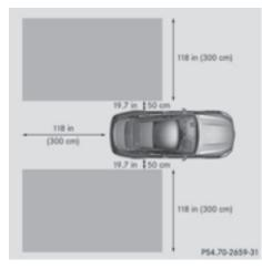
Active Blind Spot Assist monitors the area up to 10 ft (3.0 m) behind your vehicle and directly next to your vehicle, as shown in the diagram.
