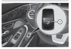
You can open and close the trunk lid from the driver's seat when the vehicle is stationary and unlocked.
