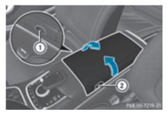
► **To open:** press button ① or ② and fold the armrest to the left or right.
