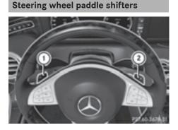
You can activate manual drive program **M** in the **E** (**C** in AMG vehicles) and **S** automatic drive programs using steering wheel paddle shifters (1) and (2) ( $\triangleright$  page 164). In manual drive program **M**, you can briefly change gear yourself by using the steering wheel paddle shifters.
