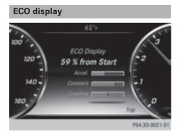
The ECO display provides feedback on how economical your driving characteristics are. The ECO display assists you in achieving the most economical driving style for the selected settings and prevailing conditions. Your driving style can significantly influence the vehicle's consumption.
