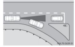
DISTRONIC PLUS does not brake for obstacles or stationary vehicles. If, for example, the detected vehicle turns a corner and reveals an obstacle or stationary vehicle, DISTRONIC PLUS will not brake for these.
