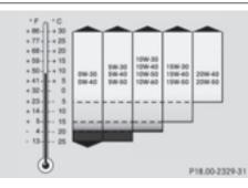
Viscosity describes the flow characteristics of a fluid. If an engine oil has a high viscosity, this means that it is thick; a low viscosity means that it is thin.
