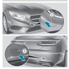
The brackets for the screw-in towing eyes are located in the bumpers. They are at the front and at the rear under covers ①.
