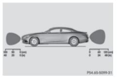
The sensors must be free from dirt, ice or slush. They can otherwise not function correctly. Clean the sensors regularly, taking care not to scratch or damage them (> page 335).
