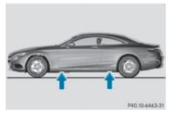
The jacking points are located just behind the front wheel housings and just in front of the rear wheel housings (arrows).
