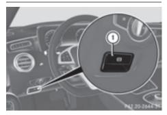
► To engage: push handle ①. When the electric parking brake is applied, the red PARK (USA only) or (②) (Canada only) indicator lamp lights up in the instrument cluster.
