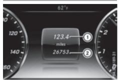
Press and hold the button on the steering wheel until the Trip menu with trip odometer (1) and odometer (2) appears.
