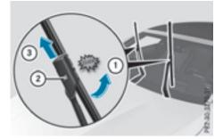
To bring the wiper blade into position to be removed: hold the wiper arm firmly with one hand. With the other hand, turn the wiper blade in the direction of arrow (1) beyond the point of resistance. The wiper blade engages in the removal position with an audible click.
