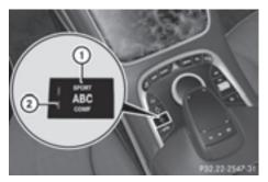
In COMFORT mode, the driving characteristics of your vehicle are especially comfortable. The steering response behavior is balanced. Select this mode if you favor a comfortable driving style.
