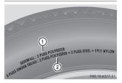
This information describes the type of tire cord and the number of layers in sidewall ① and under tire tread ②.
