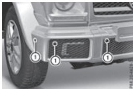
① Example: sensors in the front bumper, right-hand side
