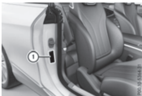
Vehicle identification plate location (example: right-hand-drive vehicle)
