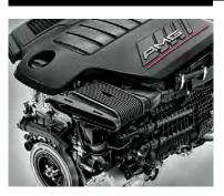
Inline-6 turbo or AMG-enhanced inline-6 turbo engine, both with EQ Boost Integrated Starter-Generator (ISG)
