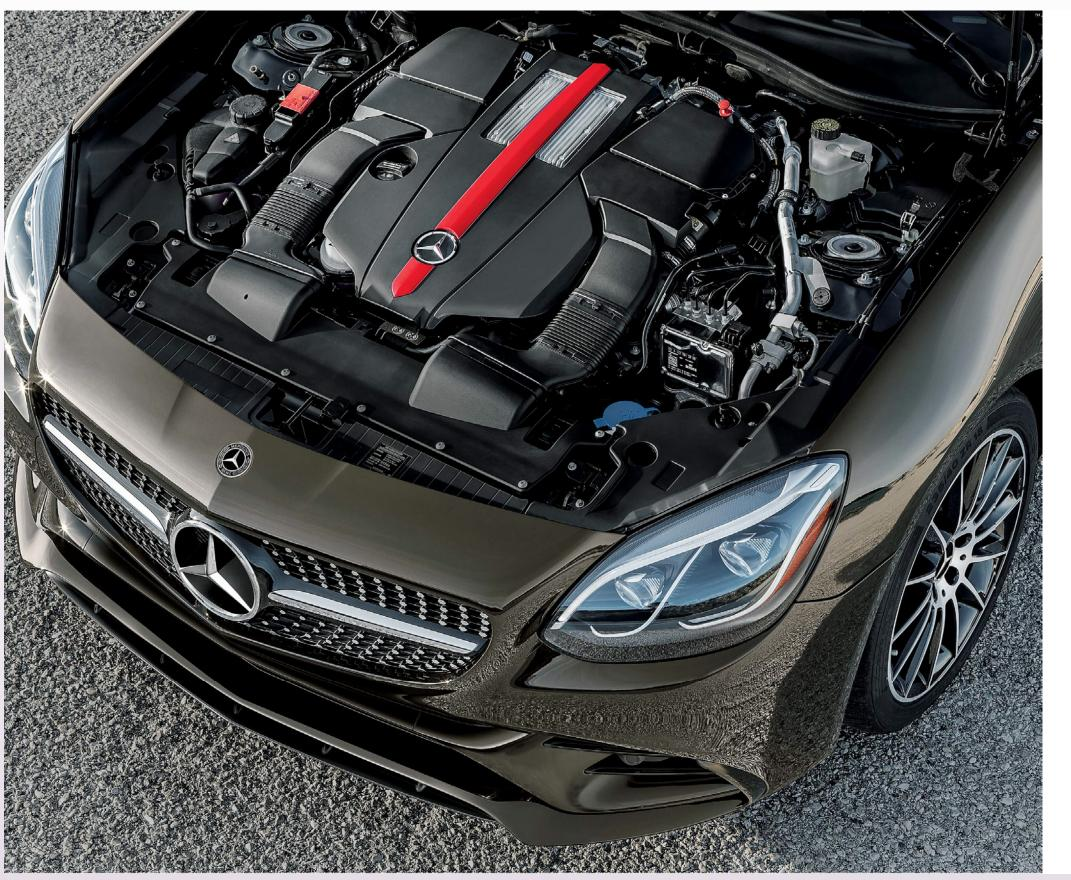
TURBOCHARGING teams with advanced Direct Injection and rapid-multispark ignition to boost power, torque and efficiency. The AMG SLC 43 is uprated to 385 hp for 2019.
