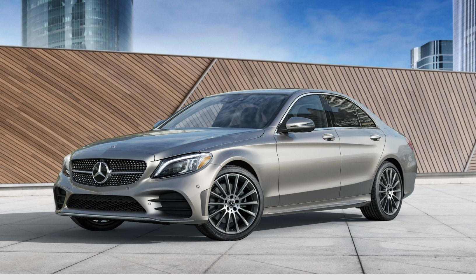
C 300 Sedan SPECIFICATIONS /ENGINE 2.0L inline-4 turbo /POWER 255 hp @ 5,800 rpm /0-60 MPH  $\rightarrow$  5.7 sec<sup>15</sup> /DRIVE rear-wheel or 4MATIC® all-wheel /SUSPENSION selective-damping /WHEELS 18" twin 5-spoke
