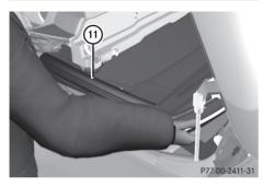
► Reach under the tip of soft top (1) in the soft-top compartment from the right-hand and left-hand sides.
