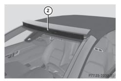
► Clean net ② of the wind deflector with a soft brush or a moist cloth. For heavier soiling, clean it with the care and cleaning agents recommended and approved by Mercedes-Benz and rinse it with clean water.
