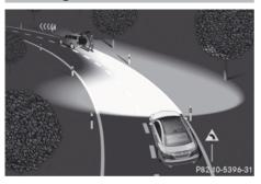
The active light function is a system that moves the headlamps according to the steering movements of the front wheels. In this way, relevant areas remain illuminated
