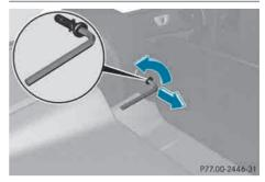
Bolts on the AIRCAP wind screen between the head restraints in the rear compartment
