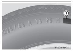
In addition to the load bearing index, load index ① may be imprinted after the letters that identify speed index ⑥ on the sidewall of the tire ( $\triangleright$  page 338).
