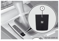
Program selector button on vehicles with the dynamic handling package
