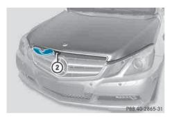
► Reach into the gap, pull hood catch handle (2) up and lift the hood. If you lift the hood approximately 15 inches (40 cm), the hood is opened and held open automatically by the gas-filled struts.
