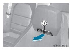
You can adjust the blower output of AIRSCARF vents (1) using the AIRSCARF button (⊳ page 112).
