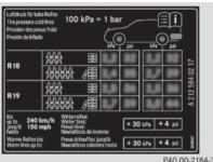
Some tire pressure tables show only the rim diameters instead of the full tire size, e.g. R18. The rim diameter is part of the tire size and can be found on the tire sidewall (⊳ page 338).
