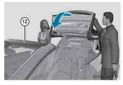
▶ Lift the soft top out of the soft-top compartment and guide it forwards in the direction of the arrow onto windshield frame ②.
