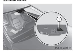
Lane Keeping Assist monitors the area in front of your vehicle by means of a camera (1) at the top of the windshield. Lane Keeping Assist detects lane markings on the road and warns you before you leave your lane unintentionally.
