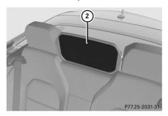
► Clean net ② of the AIRCAP wind screen with a moist cloth together with the care and cleaning agents recommended and approved by Mercedes-Benz.
