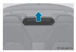
▶ Pull the AIRCAP wind screen out of the guide rails in the direction of the arrow. Make sure that you pull the AIRCAP wind screen forwards slightly when doing so.
