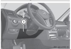
Driver's knee bag (1) deploys under the steering column. It is deployed together with the front air bags. The driver's knee bag is designed to operate together with the front air bags in frontal impacts if certain thresholds are exceeded. The driver's knee bag operates best in conjunction with correctly positioned and fastened seat belts.
