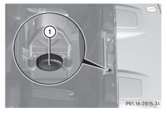
▶ Turn thumbwheel (1) in the direction of the front seat to lower the head restraints
