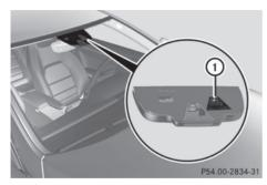
Active Lane Keeping Assist monitors the area in front of your vehicle by means of a camera ① at the top of the windshield. Active Lane Keeping Assist detects lane markings on the road and warns you before you leave your lane unintentionally. If you do not react to the warning, a lane-correcting application of the brakes can bring the vehicle back into the original lane.
