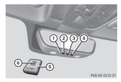
Integrated garage door opener on the rear-view
