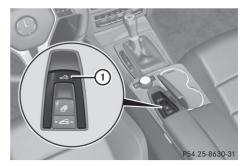
▶ To open: pull soft-top switch (1) until the entire soft top is stowed away in the trunk. The Convertible Top in Operation message appears in the multifunction display.
