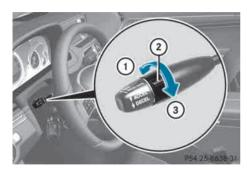
You can set the specified minimum distance for DISTRONIC PLUS by varying the time span between one and two seconds. With this function, you can set the minimum distance that DISTRONIC PLUS keeps to the vehicle in front, dependent on vehicle speed. You can see this distance in the multifunction display (> page 185).
