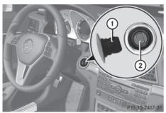
As soon as the ignition is switched on, all the indicator lamps in the instrument cluster light up. If an indicator lamp does not go out after starting the engine or lights up while driving. see (⊳ page 258).
