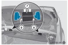
The soft-top compartment hinges are on the right-hand and left-hand side in the gap between the lid of the soft-top compartment and the trunk seal.
