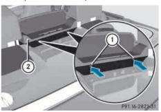
Cover (2) can only be released when the opening or closing procedure of the soft top
