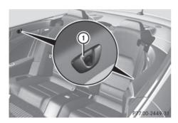
The wind screen protects against wind when driving with the soft top open. It is secured above the rear bench seats. For this reason, only the driver and the front passenger can travel in the vehicle when the wind screen is installed
