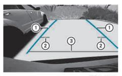
Example: information in the COMAND display Guide lines (2) and (3) show the approximate distance to the rear area. Yellow guide line (2) indicates a distance of approximately 3 ft (1 m) and red guide line (3) indicates a distance of approximately 10 in (0.25 m). The distances only apply to objects that are at ground level. Blue guide lines (1) depict the width required for the vehicle. They are used to align the vehicle with the edge of the road, e.g. the curb.
