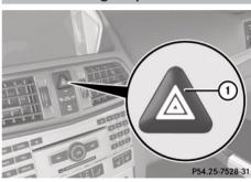
► To switch on the hazard warning lamps: press button (1).
