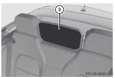
The head restraints on the rear bench seats and AIRCAP wind screen ③ move to the center position simultaneously.
