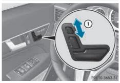
► To adjust the head restraint height: slide switch for head restraint adjustment (1) up or down in the direction of the arrow.
