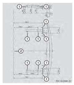
Anchorage points for the trailer tow hitch (example)
