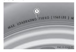
1 The actual values for tires are vehiclespecific and may deviate from the values in the illustration. Maximum tire load (1) is the maximum permissible weight for which the tire is approved.
