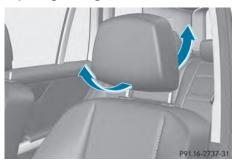
▶ Push or pull the lower edge of the head restraint in the direction of the arrow.
