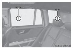
• The brackets behind B-pillar (1) are required for the cargo compartment enlargement (⊳ page 272).
