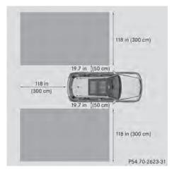
Blind Spot Assist monitors the area up to 10 ft (3m) behind your vehicle and directly next to your vehicle, as shown in the diagram. If the lanes are narrow, vehicles driving in the lane beyond the lane next to your vehicle may be indicated, especially if the vehicles are not driving in the middle of their lane. This may be the case if there are vehicles driving at the inner edge of their lanes.
