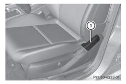
Pelvis air bags (1) deploy next to and below the outer seat cushions. They are deployed:
