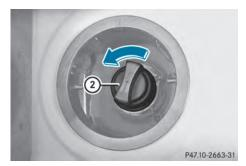
► Turn DEF filler cap (2) counter-clockwise and open it. Filler cap (2) is secured with a plastic strip.
