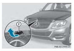
▶ Reach into the gap, pull hood catch handle ② up and lift the hood.
