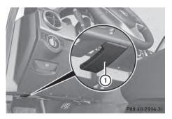
▶ Pull release lever ① on the hood. The hood is released.
