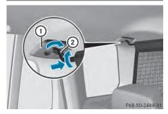
Cargo net installed behind the C-pillar
