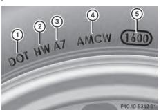
The TIN is a unique identification number. The TIN enables tire manufacturers to inform purchasers of recalls and other safety-relevant matters. It makes it possible for the purchaser to easily identify the affected tires. The TIN is made up of manufacturer identification code ②, tire size ③, tire type code ④ and manufacturing date ⑤.
