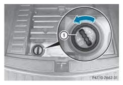
► Turn DEF cap (1) counter-clockwise and remove it.
