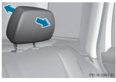
▶ Pull or push the top of the head restraint until it is in the desired position.
