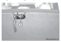
▶ Release hook (3) from the bracket on the underside of the cargo compartment floor.
