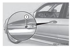
► Touch recessed sensor surface ① on the door handle until the side windows and the
