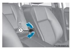
▶ Move adjustment lever (1) in the direction of the arrow until the desired backrest contour is achieved.
