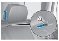
Once the head restraint is fully lowered, press release catch (1).
