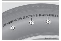
Uniform Tire Quality Grading Standards are U.S. government specifications. Their purpose is to provide drivers with uniform reliable information on tire performance data. tire manufacturers have to grade tires using three performance factors: tread wear (1), tire traction (2) and heat resistance (3). All tires sold in North America are provided with the corresponding quality class mark on the sidewall of the tire, even though these regulations do not apply to Canada.
