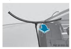
Remove the wiper blade from the retaining pin on the wiper arm in the direction of the arrow.
