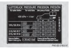
Example: tire pressure table with tire dimensions Some tire pressure tables show only the rim diameters instead of the full tire size, e.g. **R18**. The rim diameter is part of the tire size and can be found on the tire sidewall (⊳ page 346).
