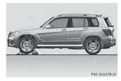
Securing the vehicle on level ground
