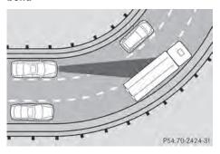
The ability of DISTRONIC PLUS to detect vehicles when cornering is limited. Your vehicle may brake unexpectedly or late.
