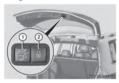
Closing and locking button (example: vehicle with EASY-PACK tailgate and KEYLESS-GO)
