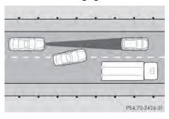
DISTRONIC PLUS has not detected the vehicle cutting in yet. The distance to this vehicle will be too short.
