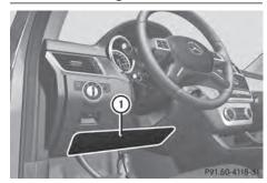
Driver's knee bag (1) deploys under the steering column. The driver's knee bag is always deployed along with the driver's front air bag. The driver's knee bag is designed to operate together with the front air bags in frontal impacts if certain thresholds are exceeded. The driver's knee bag operates best in conjunction with correctly positioned and fastened seat belts.
