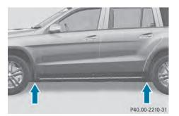
The jacking points are located just behind the front wheel housings and just in front of the rear wheel housings (arrows).
