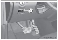
To ensure that you do not roll backwards when pulling away on an uphill slope, engage the electric parking brake.
