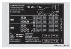
Some tire pressure tables show only the rim diameters instead of the full tire size, e.g. **R18**. The rim diameter is part of the tire size and can be found on the tire sidewall (> page 417).
