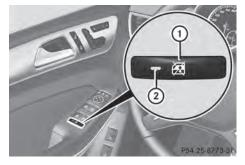
▶ To activate/deactivate: press button (1). If indicator lamp (2) is lit, operation of the rear side windows is disabled. Operation is only possible using the switches in the driver's door. If indicator lamp (2) is off, operation is possible using the switches in the rear compartment.
