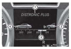
Distance display with DISTRONIC PLUS activated in the multifunction display
