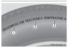
Uniform Tire Quality Grading Standards are U.S. government specifications. Their purpose is to provide drivers with uniform reliable information on tire performance data. Tire manufacturers have to grade tires using three performance factors: 1 tread wear grade, 2 traction grade and 3 temperature grade. These regulations do not apply to Canada. Nevertheless, all tires sold in North America are provided with the corresponding quality grading markings on the sidewall of the tire.
