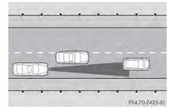
DISTRONIC PLUS may not detect vehicles traveling on a different line. The distance to the vehicle in front will be too short.
