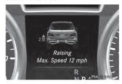
While the adjustment from off-road level 2 to off-road level 3 is taking place, you will see a message such as the following in the multifunction display: Vehicle rising Max. speed 12 mph (20 km/h).
