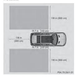
Active Blind Spot Assist monitors the area up to 10 ft (3.0 m) behind your vehicle and directly next to your vehicle, as shown in the diagram. For this purpose, Active Blind Spot Assist uses radar sensors in the rear bumper. If the lanes are narrow, vehicles driving in the lane beyond the lane next to your vehicle may be indicated, especially if the vehicles are not driving in the middle of their lane. This may be the case if there are vehicles at the inner edge of your lane.
