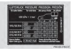
Example: tire pressure table with tire dimensions If a tire size precedes a tire pressure, the tire pressure information following is only valid for that tire size. The load conditions "partially laden" and "fully laden" are defined in the table for different numbers of occupants and amounts of luggage. The actual number of seats may differ.
