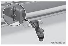
Correctly installed and secured ball coupling
