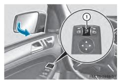
1) To fold the exterior mirrors in or out
