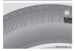
In addition to the load bearing index, load index (1) may be imprinted after the letters that identify the speed index (6) on the sidewall of the tire (> page 417).
