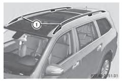
▶ Secure the roof carrier to roof rails (1). In doing so, observe the manufacturer's installation instructions.
