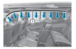
Window curtain air bags ① enhance the level of protection for the head, but not chest or arms, of the vehicle occupants on the side of the vehicle on which the impact occurs.
