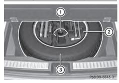
Emergency spare wheel (example: vehicle without lockable cargo compartment floor)
