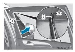
The roller sunblind can be hooked back into place should it pop out from the top of the guide rail.
