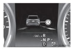
If a lane-correcting brake application occurs, display (1) appears in the multifunction display.
