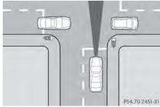
DISTRONIC PLUS may mistakenly detect vehicles that are crossing your lane. Activating DISTRONIC PLUS at traffic lights with crossing traffic, for example, could cause your vehicle to pull away unintentionally.
