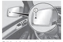
① Yellow indicator lamp/red warning lamp When Blind Spot Assist is activated, indicator lamp ① in the exterior mirrors lights up yellow at speeds of up to 20 mph (30 km/h). At speeds above 20 mph (30 km/h) the
