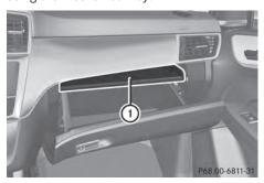
Partition ① for stowing flat objects is located in the upper section of the glove box. It can be removed to increase the stowage space in the glove box.
