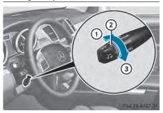
You can set the specified minimum distance for DISTRONIC PLUS by varying the time span between one and two seconds. With this function, you can set the minimum distance that DISTRONIC PLUS keeps to the vehicle in front, dependent on vehicle speed. You can
