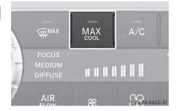
MAX COOL is only operational when the engine is running.
