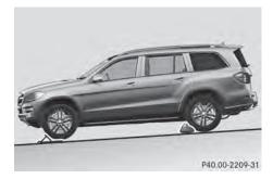
Securing the vehicle on slight downhill gradients
