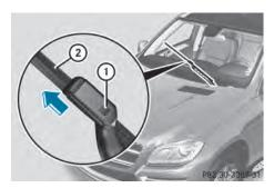
► Firmly press release knob ① and pull wiper blade ② upwards from the wiper arm in the direction of the arrow.
