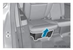
If you drop objects underneath the seats in the 3rd row, you can remove the panel in order to reach beneath the seat.
