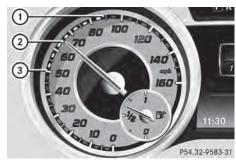
Example: DISTRONIC PLUS displays in the speedometer
