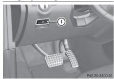
► While driving, push handle ① of the electric parking brake.
