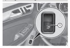
You can open and close the tailgate from the driver's seat when the vehicle is stationary and unlocked.
