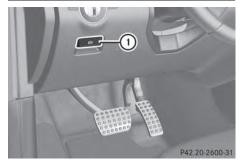
► To engage: push handle (1). When the electric parking brake is engaged, the PARK (USA only) or (P) (Canada only) red indicator lamp lights up in the instrument cluster.
