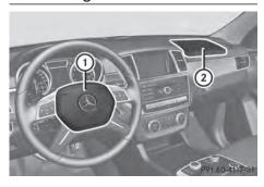
Driver's air bag ① deploys in front of the steering wheel; front-passenger front air bag ② deploys in front of and above the glove box.
