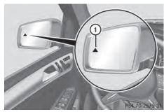
If you switch on the turn signals to change lanes and a vehicle is detected in the side monitoring range, you receive a visual and acoustic collision warning. You then hear a double warning tone and red warning lamp (1) flashes. If the turn signal remains on, detected vehicles are indicated by the flashing of red warning lamp (1). There are no further warning tones.
