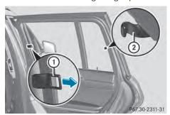
► To extend: pull the roller sunblind out by tab ① and hook it onto retainers ② at the back of the window.
