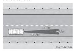
DISTRONIC PLUS has not yet detected the vehicle in front on the edge of the road, because of its narrow width. The distance to the vehicle in front will be too short.
