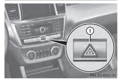
► To switch on the hazard warning lamps: press button (1).
