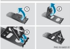
If your vehicle is equipped with a wheel chock, it can be found in the tire-change tool kit (⊳ page 264).
