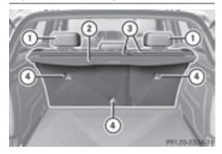
The Top Tether anchorages are located on the rear side of the rear seat backrests.
