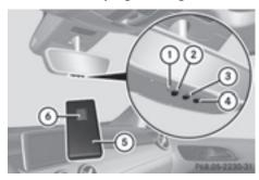
Integrated garage door opener in the rear-view mirror
