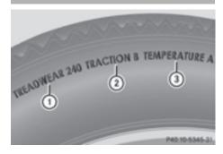
Uniform Tire Quality Grading Standards are U.S. government specifications. Their purpose is to provide drivers with uniform reliable information on tire performance data, tire manufacturers have to grade tires using three performance factors: tread wear (1), tire traction (2) and heat resistance (3). These regulations do not apply to Canada. Nevertheless, all tires sold in North America are provided with the corresponding quality grading markings on the sidewall of the tire.
