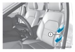
Side impact air bags (1) deploy next to the outer bolsters of the seat backrests.
