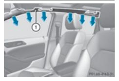
Window curtain air bags (1) are integrated into the side of the roof frame and deployed in the area from the A-pillar to the C-pillar. When deployed, the window curtain air bag enhances the level of protection for the head. However, it does not protect the chest or arms.
