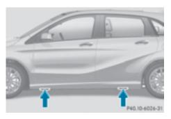
The jacking points are located just behind the wheel housings of the front wheels and just in front of the wheel housings of the rear wheels (arrows).
