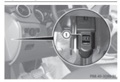
Your vehicle is equipped with a high-voltage switch-off device ① which can be used to switch off the vehicle's high-voltage electrical system.
