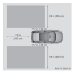
Blind Spot Assist monitors the area up to 10 ft (3.0 m) behind your vehicle and directly next to your vehicle, as shown in the diagram. For this purpose, Blind Spot Assist uses radar sensors in the rear bumper.
