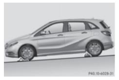
Securing the vehicle on slight downhill gradients
