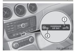
PASSENGER AIR BAG OFF indicator lamp (1) and PASSENGER AIR BAG ON indicator lamp (2) are part of the Occupant Classification System (OCS).
