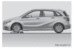
Securing the vehicle on level ground
