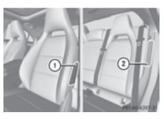
Front side impact air bags (1) and rear side impact air bags (2) deploy next to the outer seat cushions.
