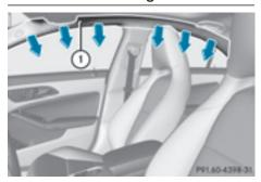
Window curtain air bags (1) enhance the level of protection for the head, but not chest or arms, of the vehicle occupants on the side of the vehicle on which the impact occurs. Window curtain air bags (1) are integrated into the side of the roof frame and deployed in the area from the A-pillar to the C-pillar.
