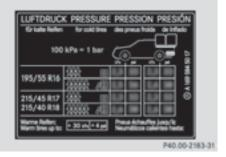
Example: tire pressure table with tire dimensions Some tire pressure tables show only the rim diameters instead of the full tire size, e.g. **R18**. Rim diameter is part of the tire size and can be found on the tire sidewall (> page 330).
