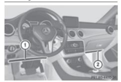
Driver's knee bag ① deploys underneath the steering column and front-passenger knee bag ② underneath the glove box. They deploy together with the front air bags. They are designed to operate together with the front air bags in frontal impacts if certain thresholds are exceeded. The knee bags operate at best in conjunction with correctly positioned and fastened seat belts.
