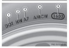
Canadian tire regulations prescribe that every new tire manufacturer or retreader has to imprint a TIN in or on the sidewall of each tire produced.
