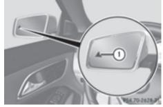
① Yellow indicator lamp/red warning lamp When Blind Spot Assist is activated, indicator lamp ① in the exterior mirrors lights up yellow at speeds of up to 20 mph (30 km/h). At speeds above 20 mph (30 km/h), the indicator lamp goes out and Blind Spot Assist is operational.
