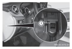
Your vehicle is equipped with a high-voltage switch-off device (1) which can be used to switch off the vehicle's high-voltage electrical system.
