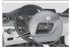
► To engage: push handle ①. When the electric parking brake is applied, the red PARK (USA only) or ⑦ (⑦) (Canada only) indicator lamp lights up in the instrument cluster.
