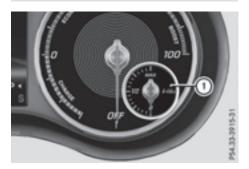
Start the drive system (▷ page 133). E-CELL display ① shows the available power of the drive system.
