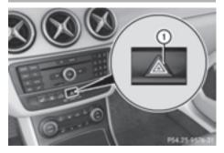
► To switch on the hazard warning lamps: press button ①.
