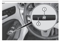
▶ To enable/disable: press button ①. If indicator lamp ② is lit, operation of the rear side windows is disabled. Operation is only possible using the switches in the driver's door. If indicator lamp ③ is off, operation is possible using the switches in the rear compartment.
