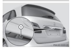
The rear view camera (1) is an optical parking and maneuvering aid. It uses guide lines to show the area behind your vehicle in the Audio/COMAND display.
