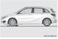
Securing the vehicle on level ground
