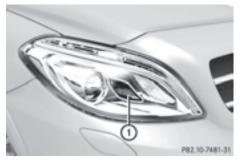
Vehicles with Bi-Xenon headlamps ① Cornering lamp: H7 55 W
