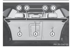
The Top Tether anchorages are located on the rear side of the rear seat backrests.
