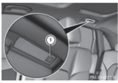
① To switch the reading lamp on/off
