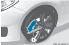
Using lug wrench ①, loosen the bolts on the wheel you wish to change by about one full turn. Do not unscrew the bolts completely.
