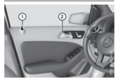
► To unlock and open a front door: pull door handle ②.
