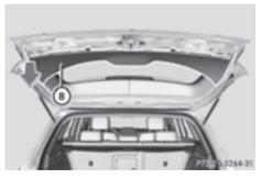
On the side where the bulb is to be replaced, unclip the remaining part of trim
