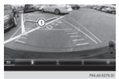
(1) Yellow guide line for the vehicle width including the exterior mirrors, for current steering wheel angle (dynamic)
