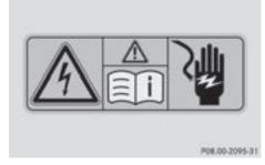
All of the vehicle's high-voltage electrical system components are marked with yellow warning stickers which warn you about high voltages. The cables of the vehicle's highvoltage electrical system are orange. When towing a vehicle after an accident, be sure to observe the following sections:
