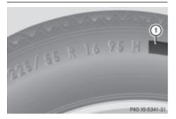
In addition to the load bearing index, load index ① may be imprinted after the letters that identify speed index ⑥ on the sidewall of the tire ( $\triangleright$  page 378).
