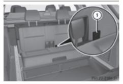
▶ Pull the seat cushion upwards by tab ① and fold it back into its original position until it engages.
