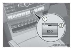
► To switch off: in drive program C, press ECO button ①.
