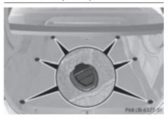
On vehicles without a through-loading feature in the rear bench seat, six plastic hooks are installed to the trunk floor.
