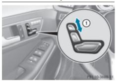
► To adjust the head restraint height: slide switch for head restraint adjustment ① up or down in the direction of the arrow.
