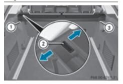
You can reach the combined cargo cover and net to install and remove it from the cargo compartment and, with the seat backrest folded forwards, from the left-hand rear door.
