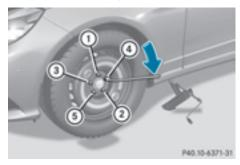
Tightening the wheel nuts (example: vehicle with an emergency spare wheel)
