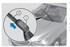
► Firmly press release knob (1) and pull wiper blade (2) upwards from the wiper arm in the direction of the arrow.
