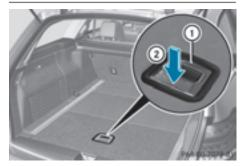
The parts of the EASY-PACK load-securing kit are contained beneath the EASY-PACK folding floor. Beneath the insert, you will find, for example, the TIREFIT kit or the emergency spare wheel and the vehicle tool kit.
