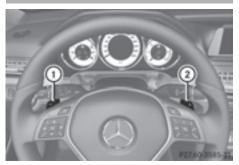
In the manual drive program, you can change gears manually using steering wheel paddle shifters (1) and (2).
