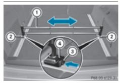
The telescopic rod can be used to secure the load against the rear seats to prevent it from moving around.
