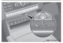
PASSENGER AIR BAG OFF indicator lamp (1) is part of the Occupant Classification System (OCS).
