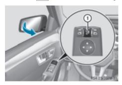
If you have switched on the Auto. Mirror Folding function and you fold in the exterior mirrors by pressing button ①, the exterior mirrors will not fold out automatically (> page 123).
