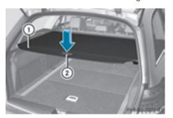
➤ To retract: unhook cargo compartment cover ① from the retainers on the left and
