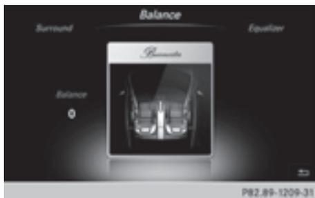
Balance adjusts the volume left and right. For the best sound, setting 0 is recommended.
