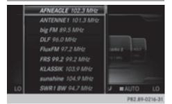
The station list is available in HD FM radio mode or HD AM radio mode. It includes all stations that can be received.
