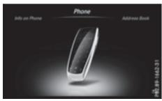
▶ Press the TEL button. If telephone mode was the last mode selected, the telephone menu appears. ► To call up the menu: press the TEL button again.
