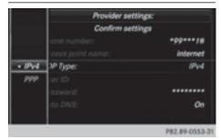
Set the access data in accordance with your data package. You can contact your mobile phone network provider to obtain the precise access data.
