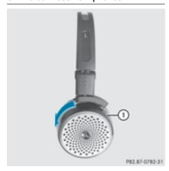
The battery compartment is located on the left headphone. The cordless headphones require two type AAA, 1.5 V batteries.
