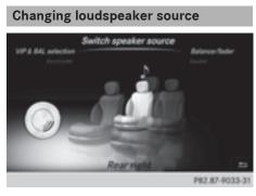
Select Sound Source specifies which seatbased media source shall be output on the speaker system.
