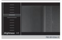
In order to manually adjust the brightness, contrast and color, the dynamic image enhancement function must be switched off.
