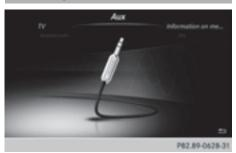
Connect an external audio source. The socket for the audio AUX jack is located in the stowage compartment in the center console.
