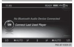
During the search for mobile phones, the connection with the Bluetooth<sup>®</sup> audio device is terminated (▷ page 142). In the Bluetooth<sup>®</sup> audio basic display (▷ page 232) you will see the No Bluetooth Audio Device Connected message and the Connect Last Used Player menu item cannot be selected.
