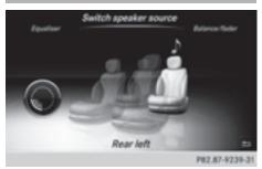
Select Sound Source specifies which seatbased media source shall be output on the speaker system. Example: a media source is being listened to using headphones in the left-hand rear seat. Rear Left must be selected in Select Sound Source if the same media source is to be listened to using the sound system.
