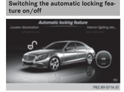
When the automatic locking feature is activated, the vehicle is locked automatically when the ignition is switched on and the vehicle is traveling faster than walking pace.
