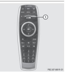
You can use the remote control to operate one of the two rear screens at a time. To do so, you must switch the remote control to the desired screen.
