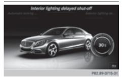
The interior lighting is activated for the duration of the delayed switch-off time when the SmartKey is removed from the ignition lock.
