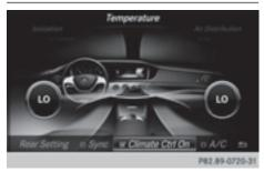
This setting is made in the bottom bar of the climate control menu.
