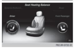
The balance function controls the distribution of heat on the seat backrest and cushion. The balance function influences the currently set heating level of the seat heating (see the vehicle Operator's Manual).
