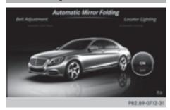
When the Automatic Mirror Folding function is activated, the exterior mirrors fold in automatically as soon as you lock the vehicle from the outside. The exterior mirrors fold out automatically again as soon as you unlock the vehicle.
