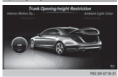
Activating the Trunk Opening-height Restriction function allows you to avoid bumping the trunk lid on a low garage ceiling, for example.
