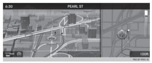
The change of direction is performed when the light-colored bar on the right drops down to 0 ft and the current vehicle position symbol has reached the white change-of-direction point. When the change of direction is completed, the map will appear in full screen mode again.
