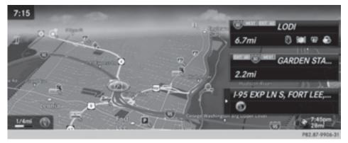
Display mode: while driving on the highway, gas stations, rest stops, rest areas and highway exits are displayed along with their immediate distances from the current vehicle position.
