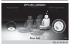
The VIP & BAL Selection setting can be used to select sound optimization for a specific seat, e.g. Rear Left.
