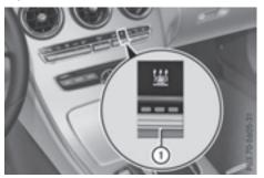
➤ To activate or deactivate "Immediate preentry climate control": press rocker switch ① up or down.
