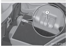
In order to prevent the trunk from being accessed by unauthorized persons, the center seat backrest can be locked using a catch. The center seat backrest can only be folded forward together with the left seat backrest.
