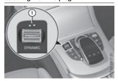
▶ Push DYNAMIC SELECT switch (1) forward or back until the desired drive program is selected
