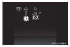
If Steering Assist and Stop&Go Pilot are activated but is not ready for a steering intervention, steering wheel symbol (1) appears in gray. If the system provides you with support by means of steering interventions, symbol (1) is shown in green.
