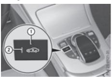
It is possible to choose between the "Normal" and "Raised" vehicle levels below a speed of 50 mph (80 km/h). Select the "Normal" setting for normal road surfaces and "Raised" for driving with snow chains or on particularly poor road surfaces. Your selection remains stored even if you remove the SmartKey from the ignition lock.
