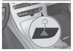
► To switch on the hazard warning lamps: press button (1). All turn signals flash. If you now switch on a
