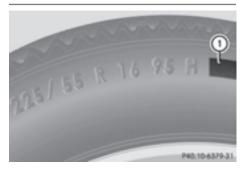
In addition to the load-bearing index, load index ① may also be imprinted on the sidewall of the tire. You will find this after the letter that identifies the speed rating ( $\triangleright$  page 374).
