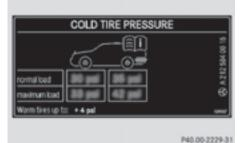
The tire pressure table contains the recommended pressures for cold tires for various operating conditions, i.e. differing load and speed conditions.
