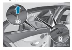
► To extend: pull the roller sunblind out by tab (1) and hook it onto retainers (2) at the top of the window.
