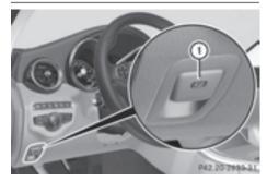
► To apply: push handle (1). When the electric parking brake is applied, the red PARK (USA only) or (P) (Canada only) indicator lamp lights up in the instrument cluster.
