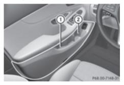
You can store items such as a rolled-up fluorescent jacket (driver's door) and the vehicle document wallet (front-passenger door) in stowage compartment (1) in the doors.
