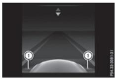
When Blind Spot Assist is activated, gray radar waves propagating backwards appear next to the vehicle in the assistance display in the multifunction display. Above a speed of 20 mph (30 km/h), the color of the radar waves in the assistance display changes to green (1). Blind Spot Assist is then ready for use.
