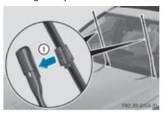
▶ Insert the new wiper blade into the wiper arm in the direction of arrow ①.
