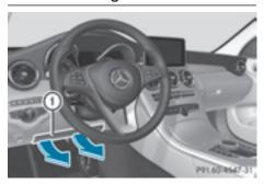
Driver's knee bag (1) deploys under the steering column. The driver's knee bag is always deployed along with the driver's front air bag. The driver's knee bag offers additional thigh, knee and lower leg protection for the occupant in the driver's seat.
