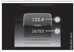
▶ Press and hold the \_\_\_\_\_ button on the steering wheel until the Trip menu with trip odometer (1) and odometer (2) appears.
