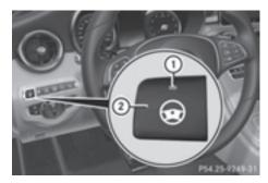
▶ Press button ②. Indicator lamp ① lights up. The DTR+: Steering Assist. On message appears in the multifunction display. Steering Assist and Stop&Go Pilot are activated.
