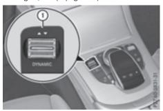
Press DYNAMIC SELECT switch ① forwards or backwards until the desired drive program is selected.
