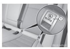
Vehicles with rear seat armrest: adjust the rear seat armrest so that LATCH-type (ISOFIX) securing rings (1) for the LATCH-type (ISOFIX) child restraint system are accessible.
