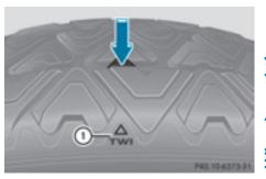
Marking (1) shows where the bar indicator (arrow) for tread wear is integrated into the tire
