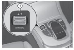
Push DYNAMIC SELECT switch ① forward or back until the desired drive program is selected.
