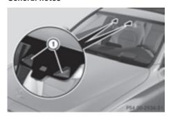
Lane Keeping Assist monitors the area in front of your vehicle by means of multifunction camera (1) which is attached behind the top of the windshield. Active Lane Keeping Assist detects lane markings on the road and can warn you before you leave your lane unintentionally.
