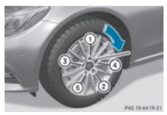
► Tighten the wheel bolts evenly in a crosswise pattern in the sequence indicated (1) to (5).
