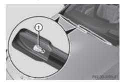
▶ Remove protective film ① of the service indicator on the tip of the wiper blade.
