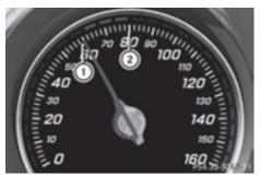
If DISTRONIC PLUS detects a vehicle in front, segments between the speed of the vehicle in front (1) and stored speed (2) light up.
