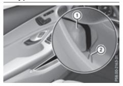
The reflective safety jackets are located in the safety jacket compartments in the stowage compartments of the front doors. There are also safety jacket compartments in the stowage compartments of the rear doors, in which reflective safety jackets can be stowed.
