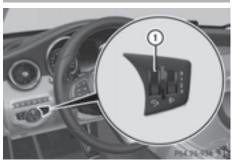
The lighting in the instrument cluster, in the displays and the controls in the vehicle interior can be adjusted using brightness control knob (1).
