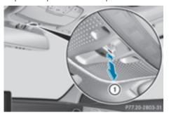
Reset the panorama roof with power tilt/sliding panel or the roller sunblinds if the panorama roof with power tilt/sliding panel or the front roller sunblind does not move smoothly.
