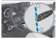
➤ To increase or reduce the set speed in 1 mph increments (Canada: 1 km/h increments): briefly press the cruise control lever up ① for a higher set speed or down ② for a lower set speed.
