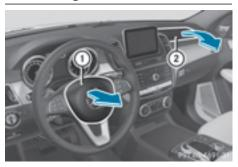
Driver's air bag ① deploys in front of the steering wheel. Front-passenger front air bag ② deploys in front of and above the glove box. When deployed, the front air bags offer additional head and thorax protection for the occupants in the front seats.
