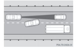
DISTRONIC PLUS has not detected the vehicle cutting in yet. The distance to this vehicle will be too short.
