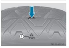
Marking (1) shows where the bar indicator (arrow) for tread wear is integrated into the tire
