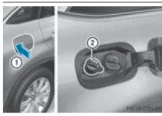
The fuel filler flap is unlocked or locked automatically when you open or close the vehicle with the SmartKey or with KEYLESS-GO.
