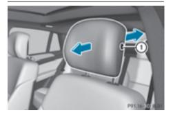
With this function you can adjust the distance between the head restraint and the back of the seat occupant's head.
