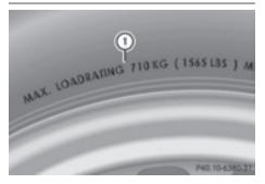
Maximum tire load ① is the maximum permissible weight for which the tire is approved. Do not overload the tires by exceeding the specified load limit. The maximum permissible load can be found on the vehicle's Tire and Loading Information placard on the B-pillar on the driver's side (> page 340).
