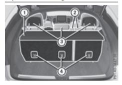
Top Tether anchorage points (4) are located on the rear side of the rear seat backrests.
