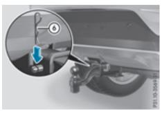
► Secure the bolt using spring cotter (6).
