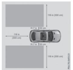
Active Blind Spot Assist monitors the area up to 10 ft (3.0 m) behind your vehicle and directly next to your vehicle, as shown in the diagram. In particular, the detection of obstacles can be impaired if:
