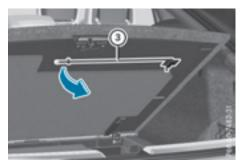
▶ Pull rod ③ from the bracket on the underside and turn it as far as it will go.
