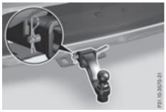
Check the ball coupling, bolt and spring cotter for correct installation.
