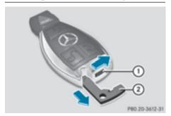
▶ Push release catch (1) in the direction of the arrow and at the same time remove mechanical key (2) from the SmartKey.
