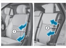
Front side impact air bags (1) and rear side impact air bags (2) deploy next to the outer bolster of the seat backrest.
