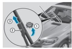
➤ To bring the wiper blade into position to be removed: hold the wiper arm firmly with one hand. With the other hand, turn the wiper blade in the direction of arrow (1) beyond the point of resistance.
