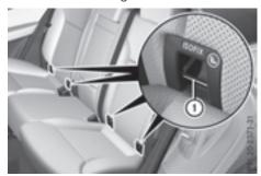
► Install the LATCH-type (ISOFIX) child restraint system on both LATCH-type (ISOFIX) securing rings (1).
