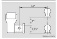
When choosing a ball coupling, the dimensions stated in the illustration must not be exceeded.
