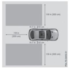
Blind Spot Assist monitors the area up to 10 ft (3 m) behind your vehicle and directly next to your vehicle, as shown in the diagram.
