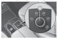
► Turn DYNAMIC SELECT controller (1) as many times as necessary until the desired drive program is selected.
