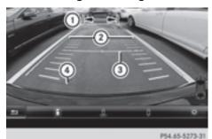
White guide line without turning the steering wheel, vehicle width including the exterior mirrors (static)
