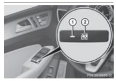
▶ To activate/deactivate: press button ②. If indicator lamp (1) is lit, operation of the rear side windows is disabled. Operation is only possible using the switches in the driver's door. If indicator lamp (1) is off, operation is possible using the switches in the rear compartment.
