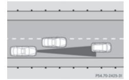
DISTRONIC PLUS may not detect vehicles traveling on a different line. The distance to the vehicle in front will be too short.
