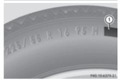
In addition to the load bearing index, load index 1 may be imprinted after the letters that identify speed index 6 on the sidewall of the tire ( $\triangleright$  page 346).
