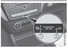
PASSENGER AIR BAG ON indicator lamp ① and PASSENGER AIR BAG OFF indicator lamp ② are part of the Occupant Classification System (OCS).
