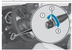
You can set the specified minimum distance for DISTRONIC PLUS by varying the time span between one and two seconds. With this function, you can set the minimum distance that DISTRONIC PLUS keeps to the vehicle in front, dependent on vehicle speed. You can see this distance in the multifunction display (> page 175).
