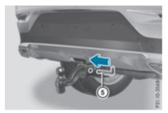
▶ Slide bolt ⑤ into the hole in the ball coupling recess and the ball coupling to the stop.
