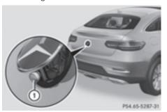
(1) Camera (1) in the rear is integrated into the emblem and thus protected from dust and dirt. The emblem opens when the 360° camera is activated. Observe the notes on cleaning (> page 312).
