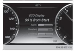
The ECO display provides feedback on how economical your driving characteristics are. The ECO display assists you in achieving the most economical driving style for the selected settings and prevailing conditions. Your driving style can significantly influence the vehicle's consumption.
