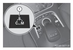
► Mercedes-AMG vehicles: press program selector button ① repeatedly until the letter for the desired drive program appears in the multifunction display.
