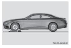
➤ On level ground: place chocks or other suitable items under the front and rear of the wheel that is diagonally opposite the wheel you wish to change.
