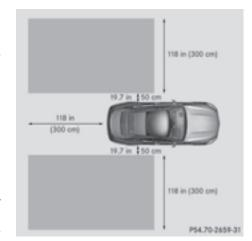
Active Blind Spot Assist monitors the area up to 10 ft (3.0 m) behind your vehicle and directly next to your vehicle, as shown in the diagram.
