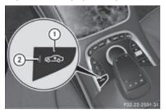
While driving, the raised level can only be selected at speeds of under 75 mph (120 km/h).
