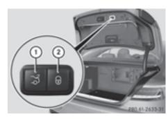
► Press and release closing button ① on the trunk lid.
