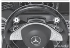
You can activate manual drive program  $\mathbf{M}$  in the  $\mathbf{E}$  ( $\mathbf{C}$  in AMG vehicles) and  $\mathbf{S}$  automatic drive programs using steering wheel paddle shifters ① and ② ( $\triangleright$  page 164). In manual drive program  $\mathbf{M}$ , you can briefly change gear yourself by using the steering wheel paddle shifters.
