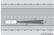
DISTRONIC PLUS has not yet detected the vehicle in front on the edge of the road, because of its narrow width. The distance to the vehicle in front will be too short.
