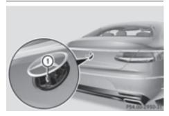
Rear view camera (1) is under a flap in the trunk lid.
