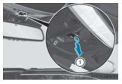
Reset the roller sunblind if it does not operate smoothly.
