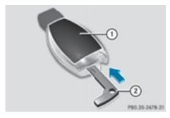
▶ Press mechanical key ② into the opening in the SmartKey in the direction of the arrow until battery compartment cover ①
