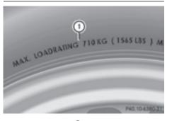
Maximum tire load ① is the maximum permissible weight for which the tire is approved. Do not overload the tires by exceeding the specified load limit. The maximum permissible load can be found on the vehicle's Tire and Loading Information placard on the B-pillar on the driver's side (▷ page 372).
