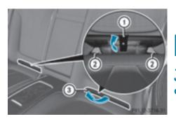
LATCH-type (ISOFIX) securing rings ② on the rear seats are covered by folding upholstered lining ③ with Velcro fastening.
