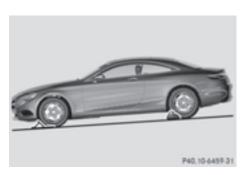
➤ On light downhill gradients: place chocks or other suitable items in front of the wheels of the front and rear axle.
