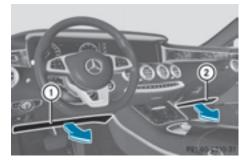
Driver's knee bag (1) deploys under the steering column and front-passenger knee bag (2) under the glove box. The driver's and frontpassenger knee bags are triggered together with the front air bags.
