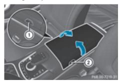
► **To open:** press button ① or ② and fold the armrest to the left or right.
