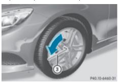
► Using lug wrench ③, loosen the bolts on the wheel you wish to change by about one full turn. Do not unscrew the bolts completely.
