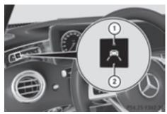
▶ Press button ②. Indicator lamp ① lights up. The Lane Keeping Assist On message appears in the multifunction display. If all conditions have been satisfied, a warning or steering intervention may be made.
