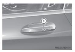
► Touch recessed sensor surface ① on the door handle until the side windows are fully closed.
