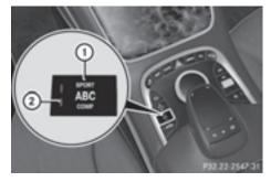
In COMFORT mode, the driving characteristics of your vehicle are especially comforta-
