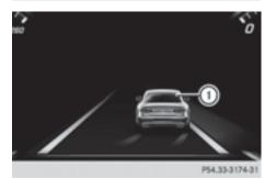
If a lane-correcting brake application occurs, display ① appears in the multifunction display. The brake application also slightly reduces vehicle speed.
