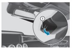
▶ Fold down the camera cover by recess (1).
