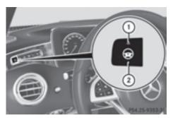
▶ Press button ②. Indicator lamp (1) lights up. The DTR+: Steering Assist. On message appears in the multifunction display. Steering Assist and Stop&Go Pilot are activated.
