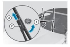
➤ To bring the wiper blade into position to be removed: hold the wiper arm firmly with one hand. With the other hand, turn the
