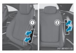
Front side impact air bags ① and rear side impact air bags ② deploy next to the outer bolster of the seat backrest.
