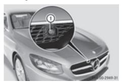
Camera lens (1) is cleaned at regular intervals by operating the windshield washer system.
