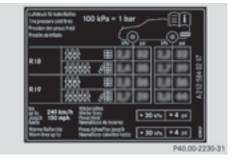
Some tire pressure tables show only the rim diameters instead of the full tire size, e.g. **R18**. The rim diameter is part of the tire size and can be found on the tire sidewall (⊳ page 377).
