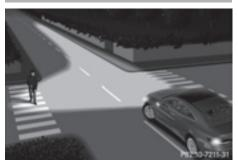
The cornering light function improves the illumination of the road over a wide angle in the direction you are turning, enabling better visibility in tight bends, for example. It can only be activated when the low-beam headlamps are switched on.
