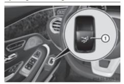
You can open and close the trunk lid from the driver's seat when the vehicle is stationary and unlocked.
