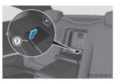
▶ Slide the tip of the mechanical key into opening (3) and turn. The lock cover is levered off.
