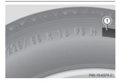
In addition to the load-bearing index, load index ① may also be imprinted on the sidewall of the tire. You will find this after the let-
