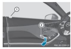
▶ Pull door handle ②. If the door is locked, locking knob (1) pops up. The door is unlocked and opens.
