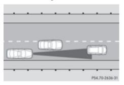
DISTRONIC PLUS may not detect vehicles traveling on a different line. The distance to the vehicle in front will be too short.
