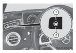
▶ Press button ②. Indicator lamp (1) goes out. The DTR+: Steering Assist. Off message appears in the multifunction display. Steering Assist and Stop&Go Pilot are deactivated.
