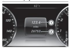
► Press and hold the ⇒ button on the steering wheel until the Trip menu with trip odometer ① and odometer ② appears.
