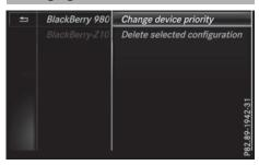
If multiple mobile phones have been enabled for Internet usage, these can be given priorities. The system then selects the mobile phone with the highest priority to establish an Internet connection.
