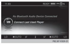
To confirm the Connect Last Used Player message in the basic display: press the controller.
