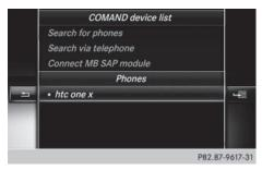
► To select a mobile phone from the device list: turn the controller and press to confirm. If the mobile phone supports the Bluetooth<sup>®</sup> PAN profile or the USB classes RNDIS, CDC/ NCM or CDC/ECM, Internet access is set up. You can use the Internet functions.
