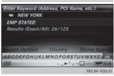
The keyword search is used to help find destinations using fragments of words. If you enable the appropriate setting in the search options, the keyword search is tolerant of errors ( $\triangleright$  page 61).
