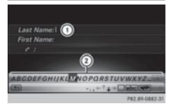
In the example, a new entry is added to the phone book ( $\triangleright$  page 103). The new entry has three input lines for entering the last name, first name and phone number. The input line for the surname is selected automatically.
