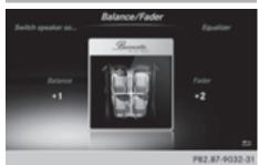
You can use balance to move the focus of the sound between left and right.
