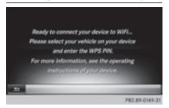
Requirement: for this type of connection, the device to be connected must support "Connect using WPS PIN".
