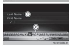
In the example, a new entry is added to the phone book ( $\triangleright$  page 103). The new entry has three input lines for entering the last name, first name and phone number. The input line for the surname is selected automatically.
