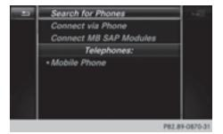
► To select a mobile phone from the device list: turn the controller and press to confirm. If the mobile phone supports the Bluetooth® PAN profile, Internet access is set up. You can use the Internet functions.
