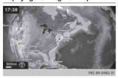
The multimedia system shows the navigation map in globe projection. This allows for a realistic map display free from distortion in all map scales.
