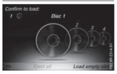
The DVD changer has a magazine with six trays. Inserting a CD/DVD into the magazine tray
