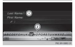
In the example, a new entry is added to the phone book ( $\triangleright$  page 100). The new entry has three input lines for entering the last name, first name and phone number. The input line for the surname is selected automatically.
