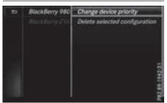
If multiple mobile phones have been enabled for Internet usage, these can be given priorities. The system then selects the mobile phone with the highest priority to establish an Internet connection.
