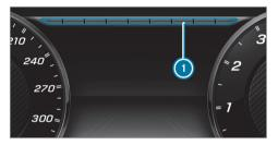
If the engine speed is too high or too low, you cannot change gear using the steering wheel paddle shifters. In this case, segments ① light up red.
