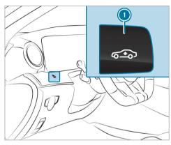
Press button ①. The vehicle is raised to the high level.
