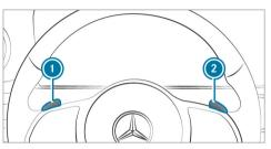
Pull steering wheel paddle shifters ① and ② and hold for half a second. If all activation conditions are fulfilled, the instrument cluster displays the DRIFT MODE Confirm: Paddle UP Cancel: Paddle DOWN message and the DRIFT warning lamp flashes. To cancel: pull steering wheel paddle shifter 1.
