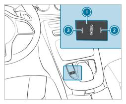
To select the Comfort suspension setting: press button () repeatedly until indicator lamps () and () go out. The AMG Suspension System COMFORT message appears in the multifunction display. In "Comfort" mode, the driving characteristics of your vehicle are comfortable.
