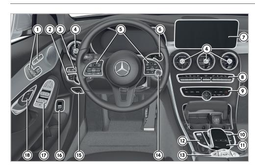
Seat ventilation Z AIRSCARF Memory function and presets 1 2 3 2 Light switch ③ Driver assistance systems Active Steering Assist
